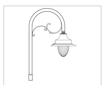
Place luminaire onto mounting pole and tighten screws evenly to ensure the luminaire is in correct alignment with the pole. Don't over tighten.
